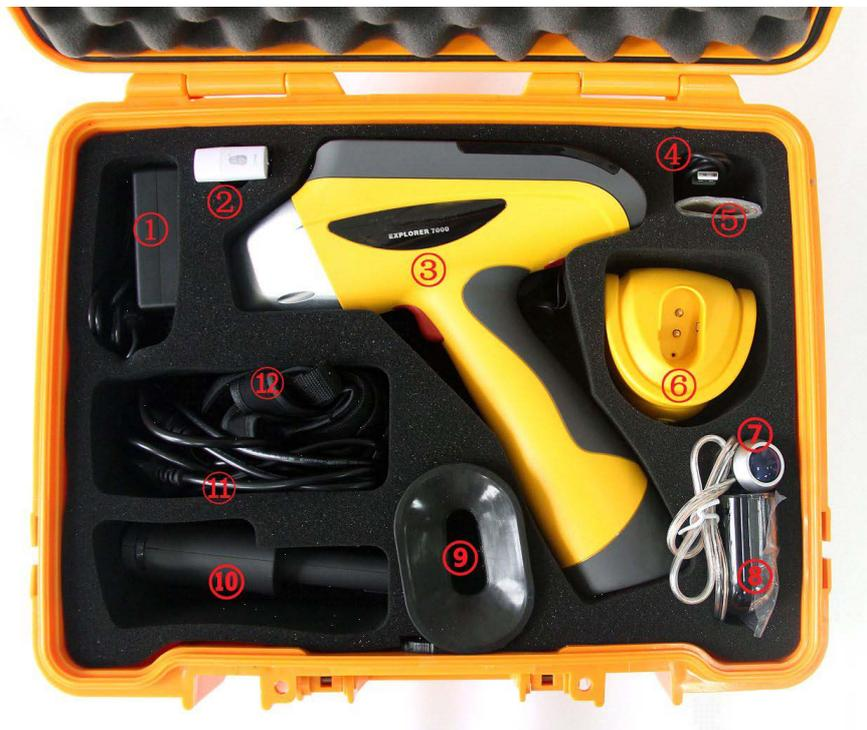
⑥ ;Adapter; ②TF reader; ③EXPLORER-9000; ④Mini USB cable; ⑤ Test membrane ①
