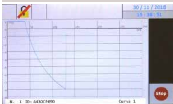
Real-time graph of the cryoscopic point measurement
