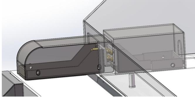
The door contact connector is a structure for supplying power to the test box door. When the door is closed, the contact is turned on, and the heating and illumination on the test box door can work normally. The door contact connector has a working voltage of 24V, which is a safe voltage and does not cause harm to people. If the politeness is dismantled, it is easy to cause the virtual contact of the contact, so that the lighting on the test box door and the heating cannot work normally.
