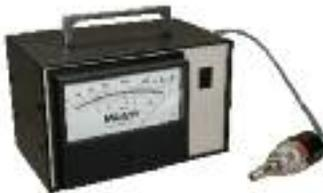
Gauges provide an accurate, reliable measurement of vacuum. Self-contained gauges with solid-state electronics for rapid response time, long life and low maintenance. Comes with a 0 to 10 VDC recorder output. The gauge sensor tubes are designed to assure maximum sensitivity over the entire vacuum range. Gauge sensor tube connected to system via 1/8" NPT thread. Each gauge comes with one sensor tube and one cable. Dimensions of 7" L x 5" D x 5.6" H (17.8 x 12.7 x 14.1); Weight 2 lbs(0.9 kg).
