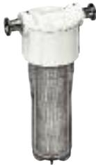
The Acid Neutralization Trap contains a large alkaline element cartridge to neutralize hydrous acids before they enter the vacuum pump. The element changes from white to bluish-transparent when spent and can be observed through the transparent trap body. Dimensions: 1420H-21, 8" W x 9" H; 1420H-20, 8" W x 13" H. (See CHEMSTAR application booklet for specific recommendations for use.)
